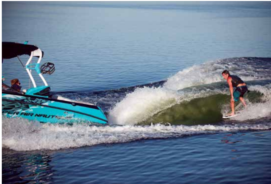
Figure 1. A typical, stern-heavy wake boat creates a large surferable wake. Photo from Pinsdaddy.
